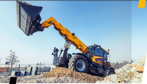
Icarus, in the New Construction Range, is the vehicle that reaches great heights: it can extend **up to 18 meters**, guaranteeing **maximum stability** thanks to the proportionally controlled independent outriggers.
